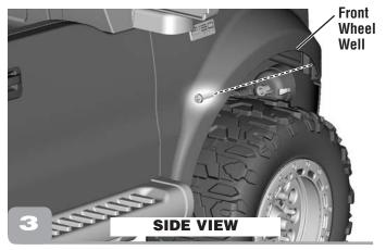
• Insert a screw through **both** front wheel wells and into the front grille. Tighten the screws.
